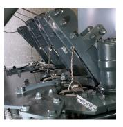
Automatic tying device ties the bales firmly, with a low consumption of steel wire.
