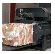
The baling channel adjusts automatically to keep the bale density high and constant.
