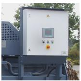
The PLC system has a touch panel, where you can set pressing force, bale length etc.
